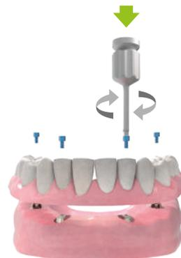
Reposition the prosthesis on the transepithelial abutments and check the fitting. Place the clinical screw using a surgical screwdriver and tighten manually. Apply 20Ncm of torque using a contra-angle screwdriver tip or a torque wrench (see torque table on page 46).
