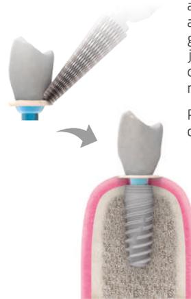
Place the abutment-restoration assembly on the implant.
