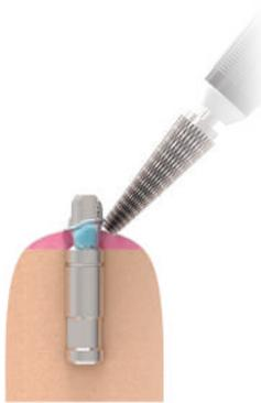
To make the final adjustments, position the abutment on the model and secure it with the laboratory screw using manual torque. Consider the preparation of margins, in aesthetic zone between 0.5 - 1 mm subgingival, in non-aesthetic areas preparation must be at the gingival or supragingival level.
