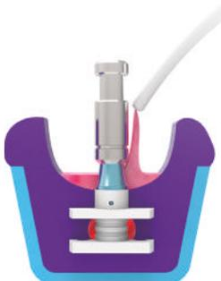
**STEP 10 - Laboratory | Impression pouring and working model**
