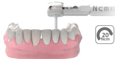
**Important note:** Do not exceed 20 Ncm to avoid screw fractures.
